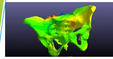
Full assembled model was simulated in Ansys. The model was constrained at the hip joints and loaded at the top of sacrum. The results did not show any stress sites in or around the the newly fitted implant
