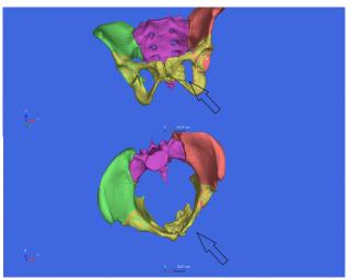
Patient had tumor on Pubic symphysis. Patient CT scan data was imported into ImageSim Software. The scan data was filtered using advanced anisotropic filtering feature in the tool. Next the filtered image was segmented and saved as STL model.
