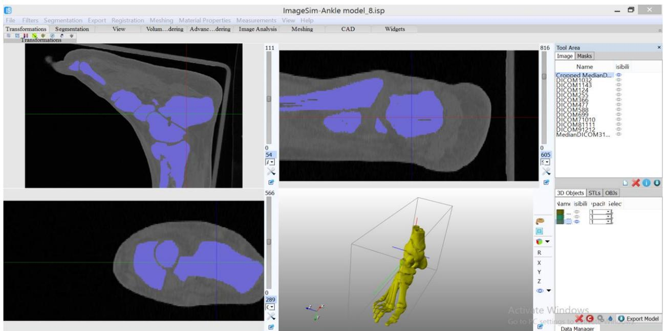
Figure [1] Patient Scan data segmented in ImageSim software
