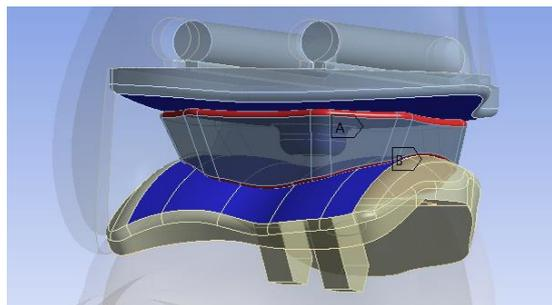
Figure [8] Implant contact Area
